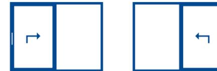
2-piece element with sliding sash and fixed glazing
